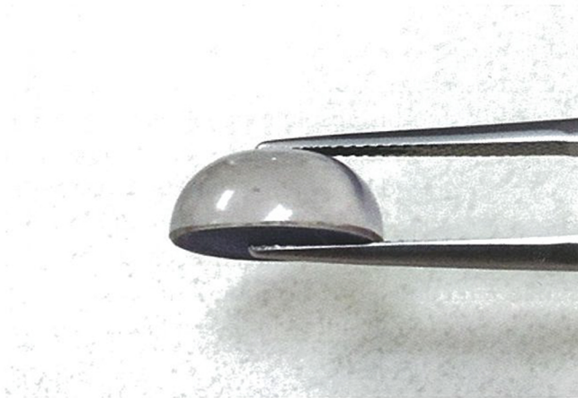
Figure 26: In profile view, it became apparent that the cabochon in Figure 25 is actually colourless. The blue colour viewed face-up is due to a coating on the bottom of the cabochon. Photo by Kelly Kramer.
