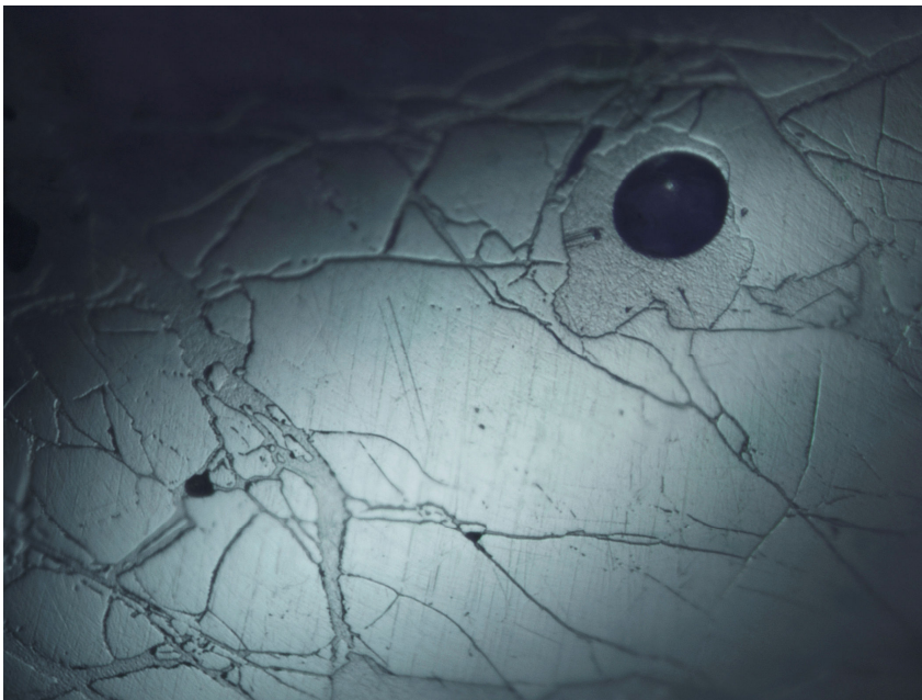
Figure 3: With overhead, reflected light the surface of these stones were seen to be traversed by an extensive network of fractures, broad seams, parting planes and cavities that were filled with a high lead-content glass which is very close in refractive index to the host corundum. Photomicrograph by Christopher P. Smith, 75x.
